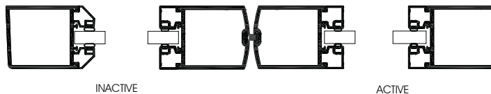
DRGS-14 OFFSET HUNG DOOR 1/4" SQUARE GLASS STOP
